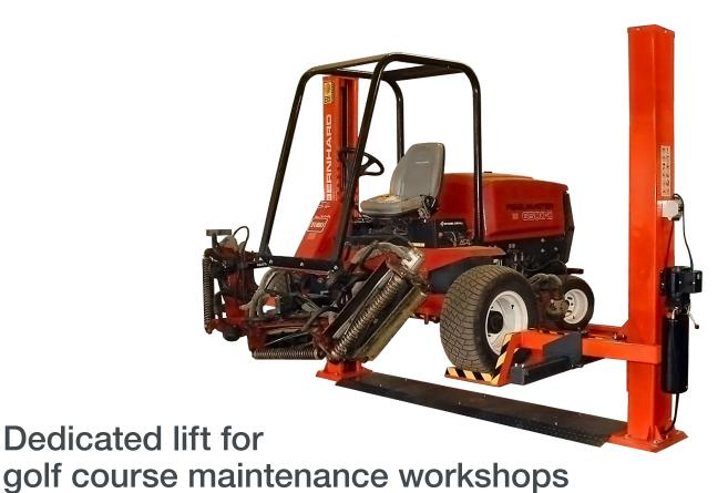
Specification Metric Imperial Capacity 2500 Kg 5511.5 lbs Lifting height (max) 1700 mm 67" Lifting time Up 50 s; down 48 s Up 50 s; down 48 s 2.2 kW 2.95 HP Motor 240 V 240 V Power 42.1" to 78.7" Wheelbase range 1070 mm to 2000 mm Wheel track range) 1250 mm to 2500 mm 49.21" to 98.4"
